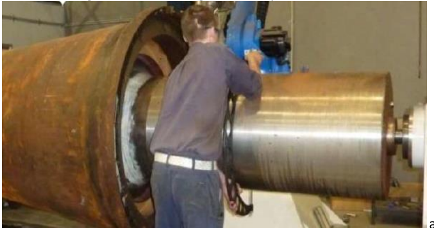
Picture 2 – large drive shaft being serviced by Laserbond
