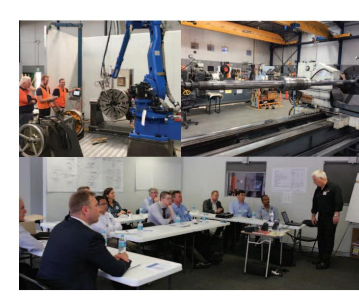
LaserBond designs and manufactures its own high power laser cladding cells for the heavy industrial market. These usually include patent pending technology and innovations for an efficient, integrated, high capacity system that includes close-coupled laser diode power units, multi-axis robotic cladding and component handling, improved safety and an ancillary equipment package.
