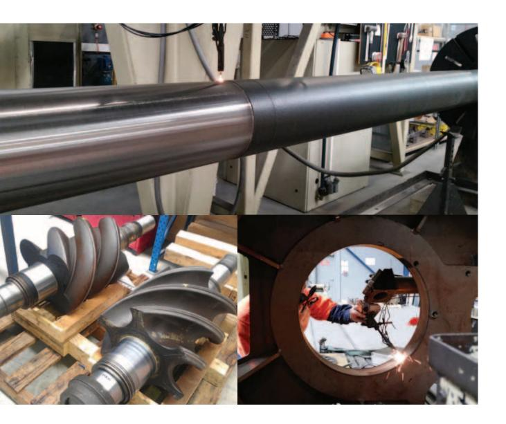
Application of LaserBond's surface engineering expertise delivers game-changing products and new processes. The development of our new laser deposition method enables fast cladding of thinner films of tailored wear resistant non-homogeneous alloys. These can be applied internally and externally to suit many end-use applications. This game-changing thinking delivers economic hard-chrome
