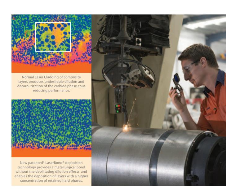
Our R&D team invented a new method for depositing thin, metallurgically bonded coatings to structural substrate metals using laser systems. Working with scientists at the Australian Synchrotron the outcomes are shown (above) by way of some advanced imaging obtained using the Scanning X-ray Fluorescence Beamline Microscopy. It has provided unprecedented visual proof that LaserBond's new method is far superior to that which had been used previously. This
