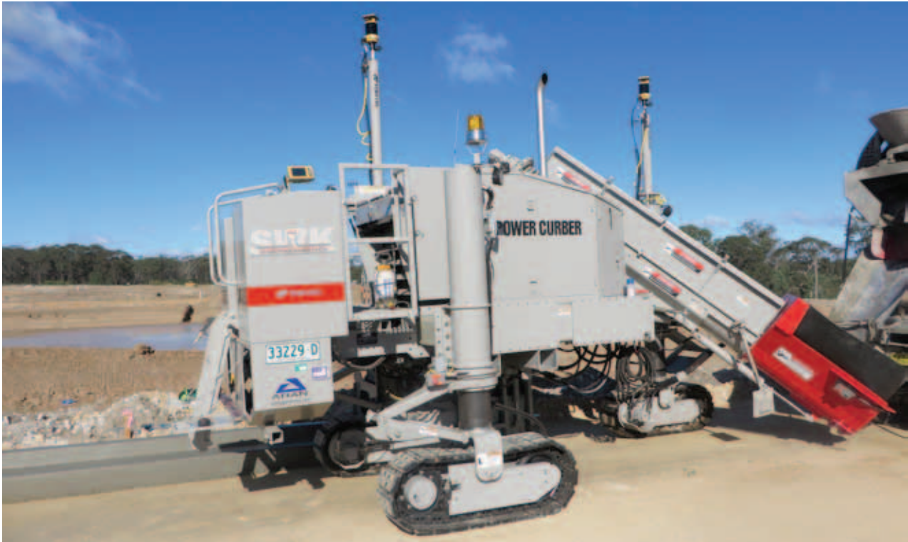
Concrete slip forming machines allow the continuous in-situ pouring of concrete structures. Typical applications include kerbing and roadside barriers. An important part of the machines is the feed auger which continuously elevates the wet concrete into the mould.
