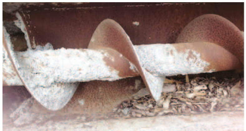
Worn standard auger conveyor after 400 hours. Note large gap from outside of flights to chute.
