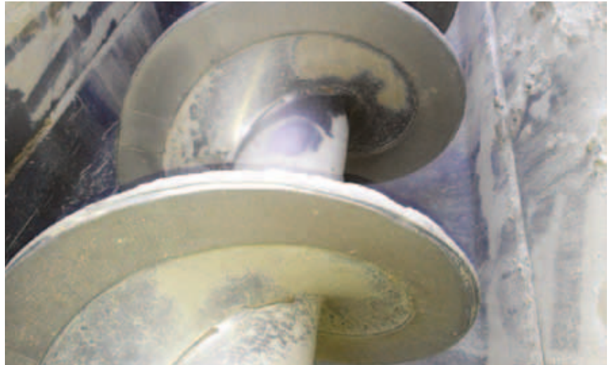
LaserBond® clad auger after 1900 hours of operation. Note outside diameter is hardly worn.
