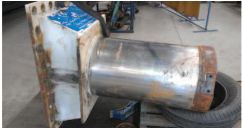
Ram component showing the high wear area to be machined, clad and superfinished.
