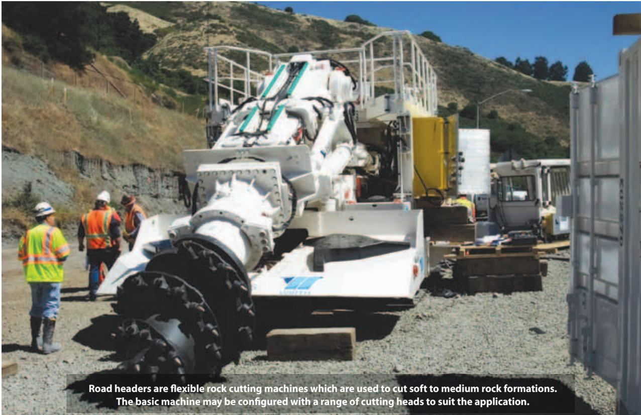
Road headers are flexible rock cutting machines which are used to cut soft to medium rock formations. The basic machine may be configured with a range of cutting heads to suit the application.
