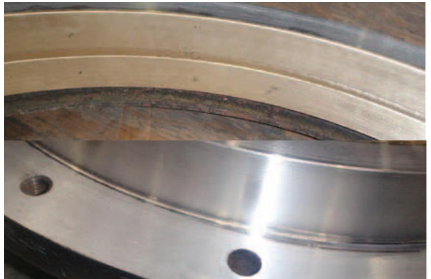
Boom guide ring inner and outer surfaces after machining.
