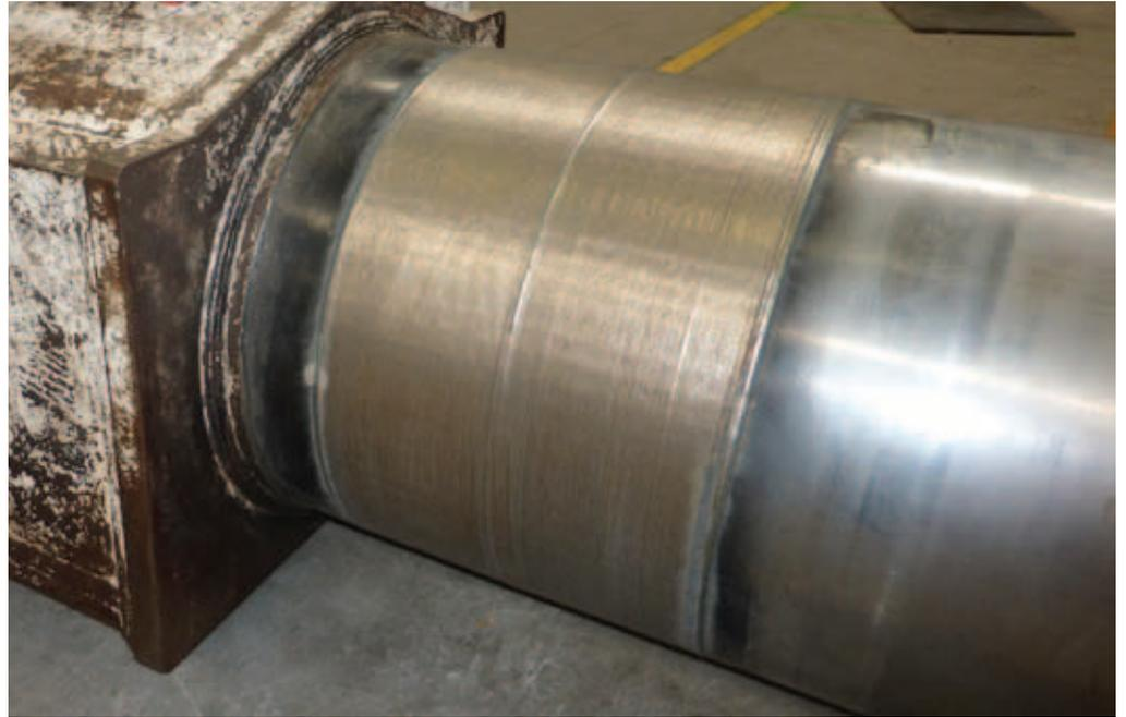
Cutter boom ram finished after LaserBond® cladding, machining and blending a superfinished surface over a 300mm area.
