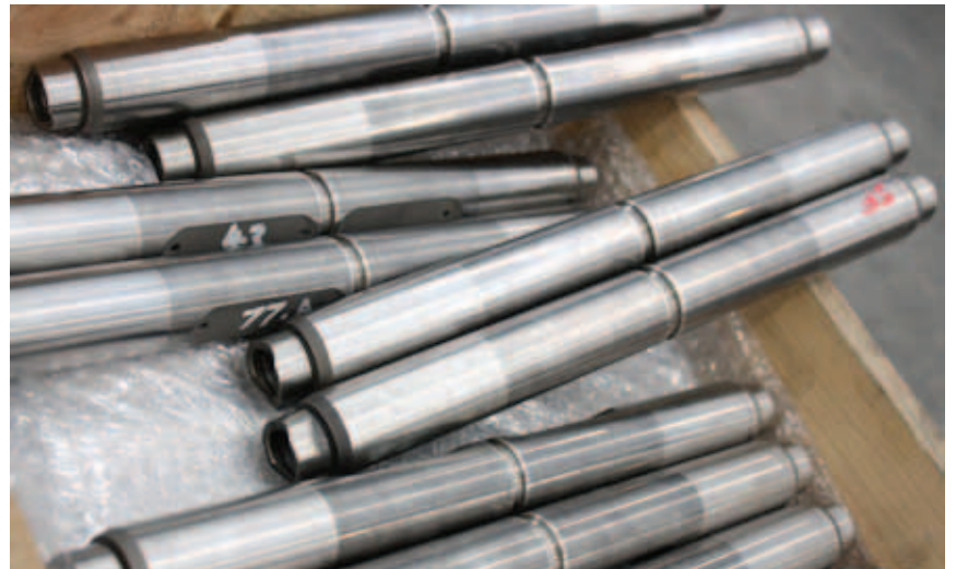
Reamer pins are machined, heat treated and HP-HVOF clad to provide high quality and economic products suited for abrasive duty.
