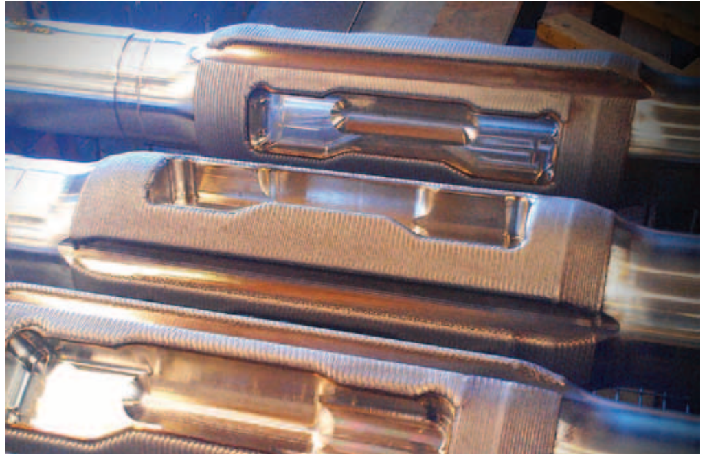
LaserBond cladding of the main reamer body reduces wear from erosion of the high velocity drilling cuttings which accelerate through the narrow annulus of the reaming unit.
