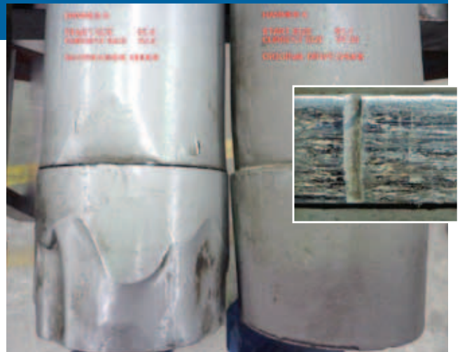
Comparison of wear after 3500m from an industry leading brand (which was scrapped) and the LaserBond Hammer which went on for another 8000m. Inset: internal galling and crack initiation.
