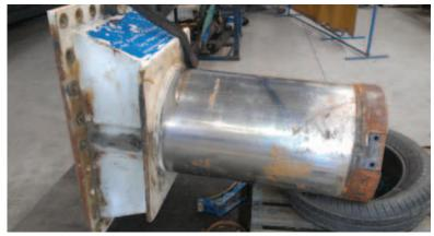
Ram component showing the high wear area to be machined, clad and superfinished.
