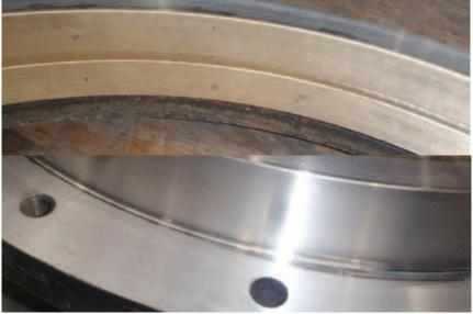
Boom guide ring inner and outer surfaces after machining.
