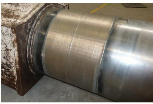
Cutter boom ram finished after LaserBond® cladding, machining and blending a superfinished surface over a 300mm area.
